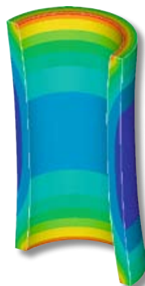
Finite-Elemente-Modell eines elektroaktiven Elastomeraktors. Finite element model of an electroactive polymer actuator.
