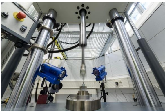
Dynamic analysis of a plastic sample with the prototyped high-speed testing machine. Photo: Fraunhofer LBF
