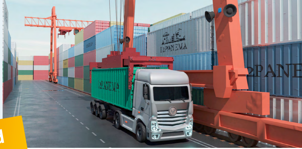
Speakers on the crane reduce the amount of noise when setting the container down on the truck by transmitting adaptively calculated inverted noise. (©Fraunhofer IML)
