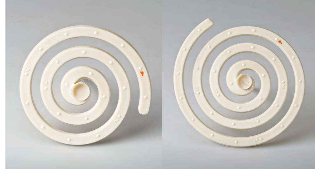
Improved flowability in the spiral test of the polyamide 6 blend (right) compared to commercially available thermally conductive polyamide 6 (left)
