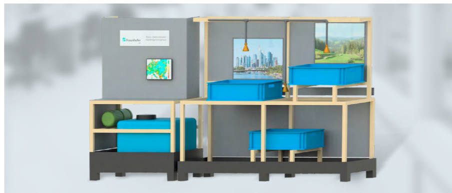
System to simulate heavy rainfall events.
