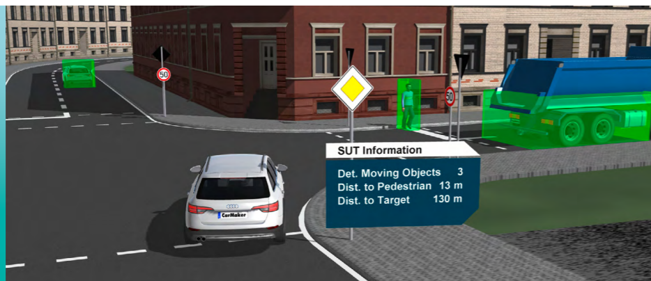
Simulation-based testing makes it possible to evaluate the performance of automated driving functions in a wide range of traffic situations at low cost and risk. (© IPG Automotive GmbH)
