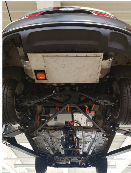
HyPowerRange energy storage system in the test vehicle.
