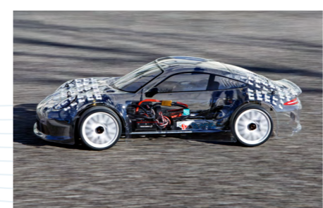
Exemplary implementation of vibro-acoustic metamaterials on a vehicle model.
