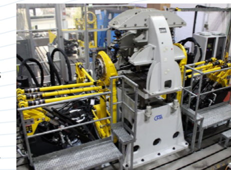
Road simulator for validating entire vehicle frames.
