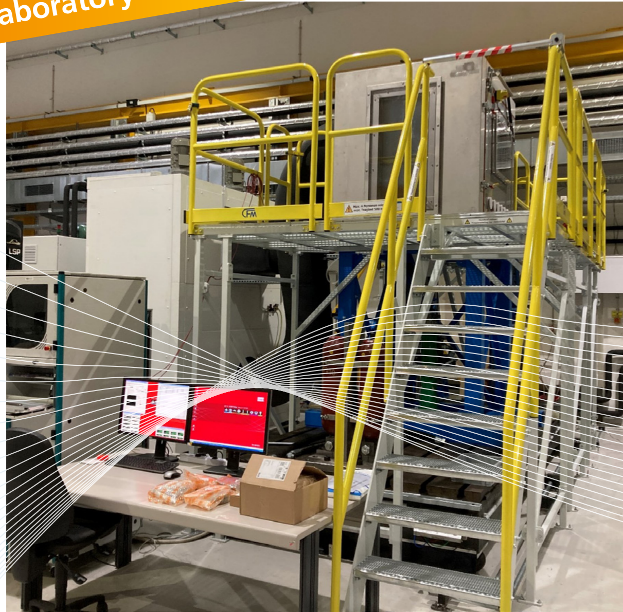
Lab facility for validating active suspension/damper systems and air suspension systems.
