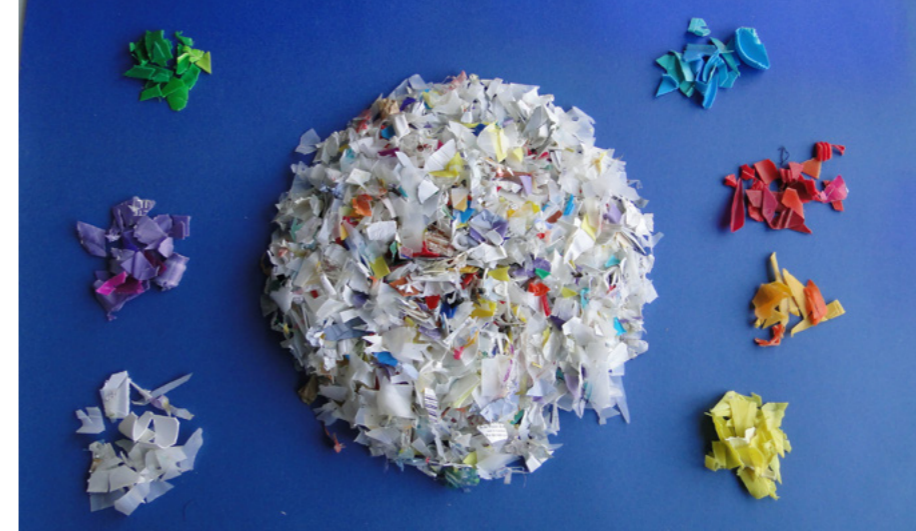
Sorted and washed post-consumer polyethylene waste broken down into flakes.
