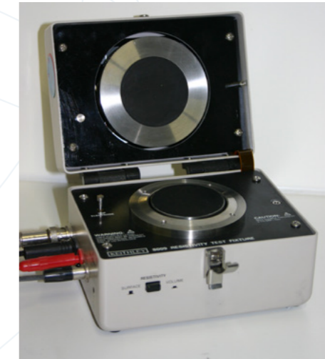
Measuring cell for measuring volume conductivity and surface conductivity of plastic films and plates.
