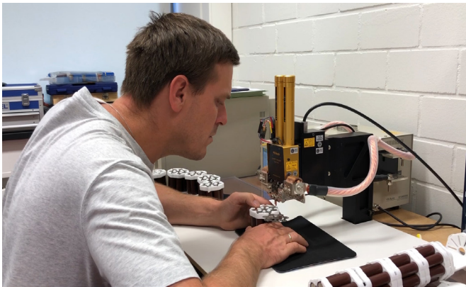
Resistance spot welding of Li-ion cells at Fraunhofer LBF
