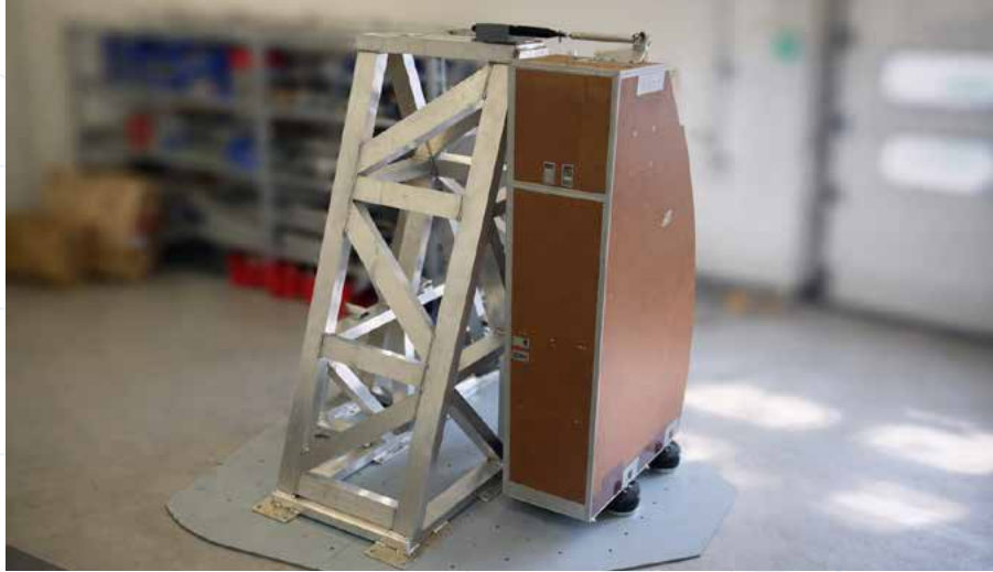
Test environment with the cabin monument on the Multi-Axial Vibration Table (MAST) as a real system on a monument table.
