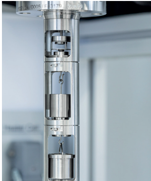
Sensor of the micro balance for hydrogen absorption testing.
