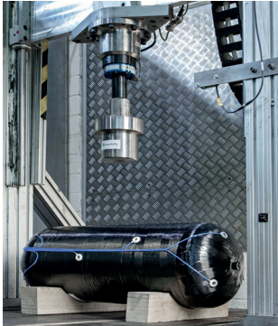
Test rig for the characterisation and validation of the AE sensors applied on H_2 tank.
