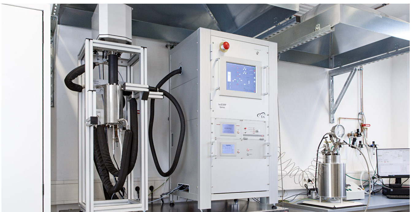
Test environment for hydrogen absorption of materials (weight up to 25 g).
