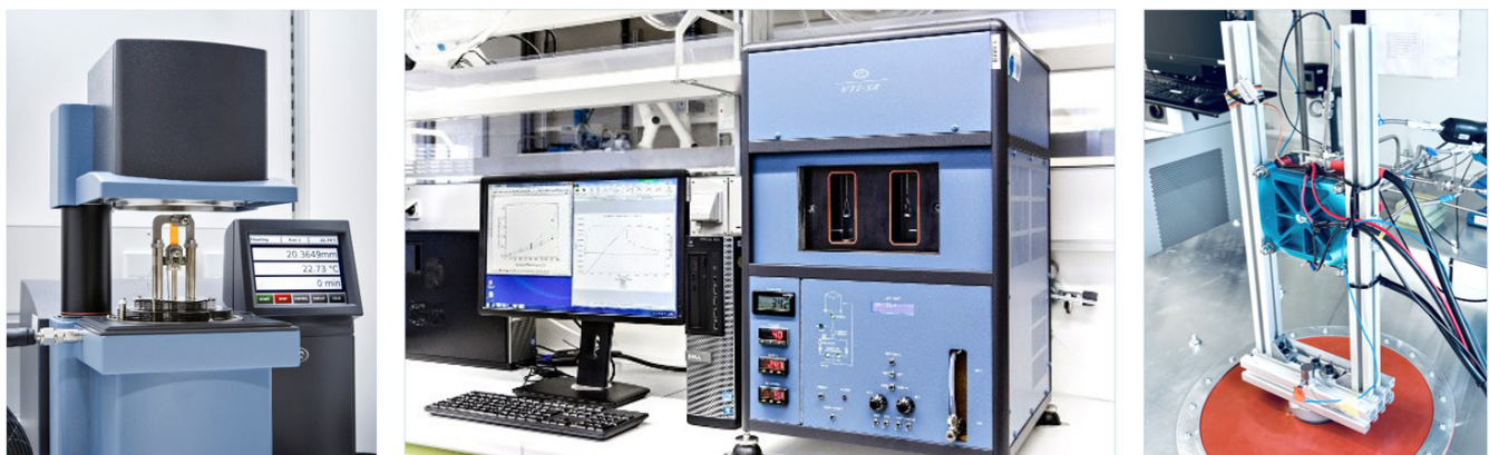
Experimental methods for fuel cell testing, including dynamic mechanical analysis (DMA), sorption analysis (SA) and single cell testing under vibration to assess mechanical behavior and transport properties.
