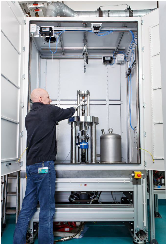
Test rig for measurements under H 2 atmosphere up to 100 bar pressure.
