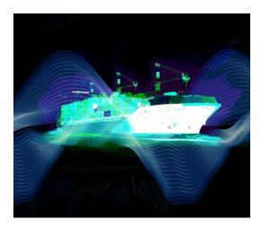
Ships undergo enormous vibrations. These are triggered by the powerful diesel engines. The vibrations are disturbing and damage components. Adaptronic systems help to reduce the vibrations. At the SMM, the Fraunhofer LBF is presenting a simulation software for these systems. Photo: Fraunhofer LBF
