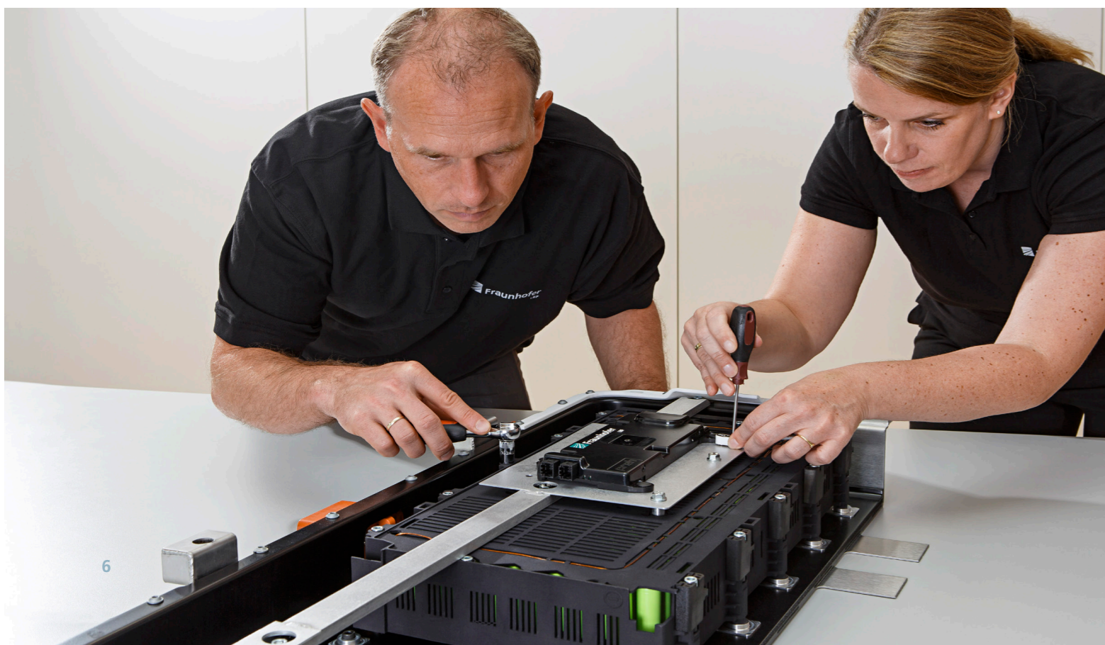
Fig. 2: Dismantling the batteries of electric vehicles for a 2nd-life application.
