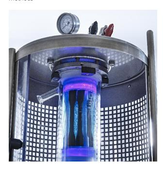
Material under pressure: Lifetime analysis under alkaline or acidic electrolyzer conditions at elevated pressure and temperature at Fraunhofer LBF. Photo: Fraunhofer LBF, Raapke
