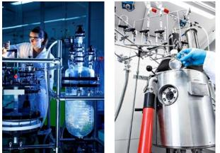
(Left): With Filtration, products are isolated and purified. (Right): A 20-liter autoclave enables syntheses under inert conditions as well as in a vacuum or under increased pressures. Photos: Raapke/Fraunhofer LBF
