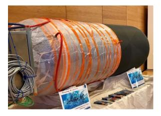
"CFRP Booster Housing," manufactured using a digitally-controlled vacuum infusion process. Photo: Fraunhofer LBF
